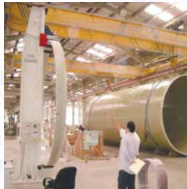
Electro-mechanical Stiffness Testing Machine Diameter Range DN250 - DN4000
