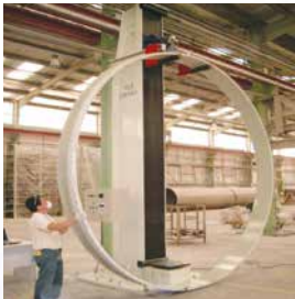
Electro-mechanical Stiffness Testing Machine Diameter Range DN250 - DN4000
