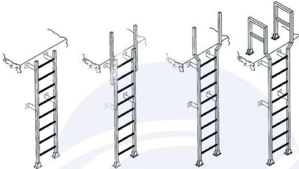
Ladder 400mm    Ladder with 600mm Walk-thru    Ladder with 750mm Walk-thru    Ladder with walk-thru and handrail connections to floor
