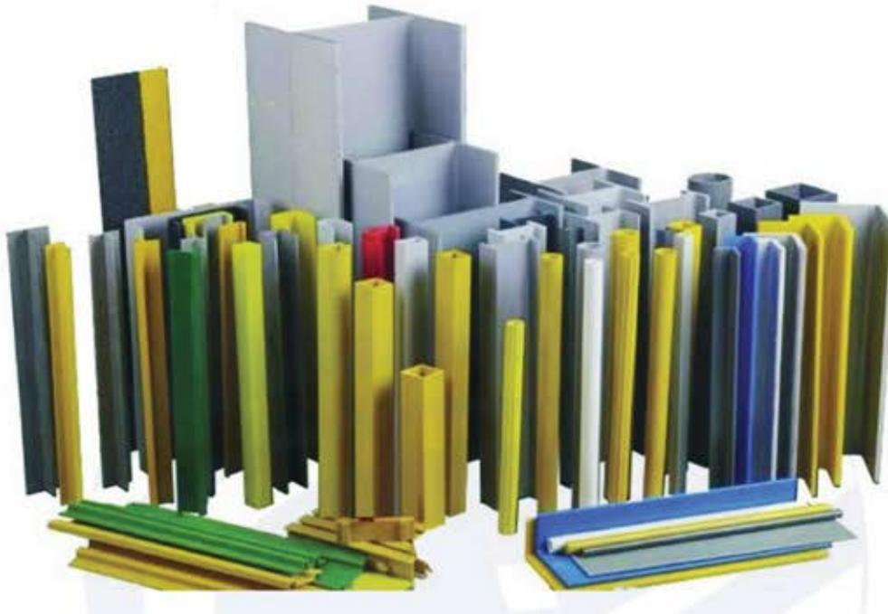
FRP pultruded profiles (structural shapes) are manufactured with the pultrusion process. Glass mat and roving are drawn through resin bath and pulled through a heated die to form the desired shape. GOODWIN pultruded profiles are available in a wide variety of shapes, including I beam, equal angle, channel, square tube, round tube, and so on. They are dimensionally stable and easy to install.
