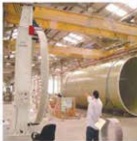
Electro-mechanical Stiffness Testing Machine Diameter Range DN250 - DN4000
