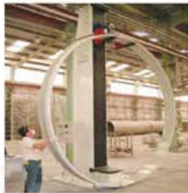
Electro-mechanical Stiffness Testing Machine Diameter Range DN250 - DN4000
