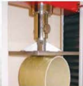
Stiffness Testing Conform to standard ISO 7685 & ASTM D2412
