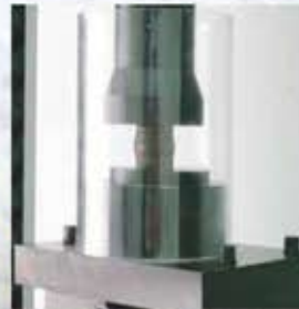
Compression Testing Conform to standard ASTM D695
