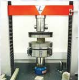
Compression Testing Conform to standard ASTM D695
