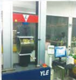
Stiffness Testing Conform to standard ISO 7685 & ASTM D2412
